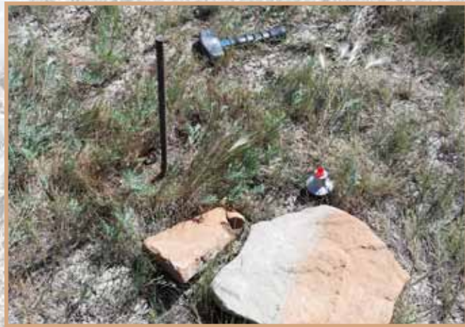
Photo 4: Rebar set at recovered portion of stone monument
