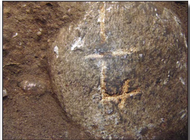
Figure 4 - Original quarter corner stone found 14" below ground surface, with chiseled markings.
