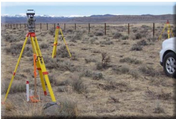
SETTING REFERENCE MONUMENTS FOR HARN STATION "L49", PID OW0104
