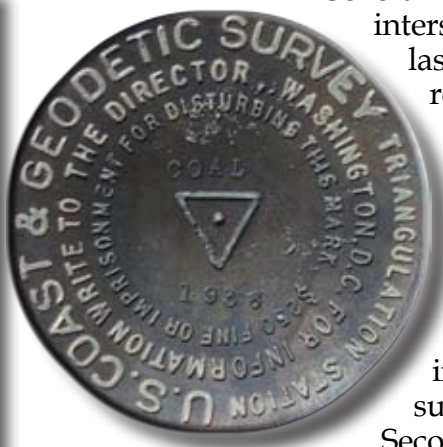
NSRS STATION COAL, PID OW0249, TYPICAL DISK IN ROCK OUTCROP
