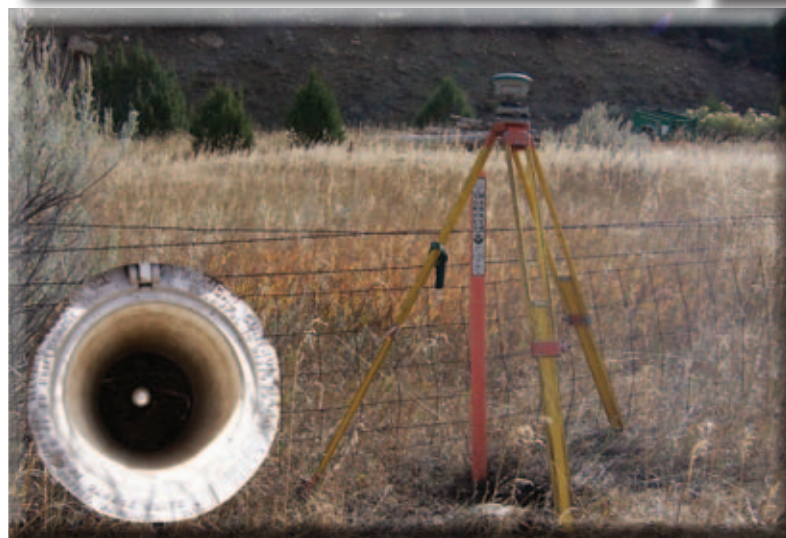
NSRS (BM) STATION "V 327", PID OW0216 IS A TYPICAL ROD IN BOX WITH COVER ALONG U.S. HIGHWAY 20 IN THE WIND RIVER CANYON
