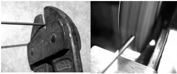
Cutting the rod with bolt cutters
