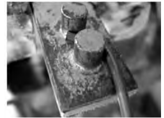
Begin the bend keeping it tight against the post
